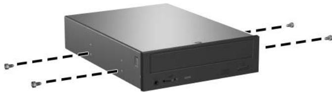
Installing Guide Screws in the Optical Drive
