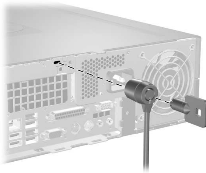
Installing a Cable Lock
