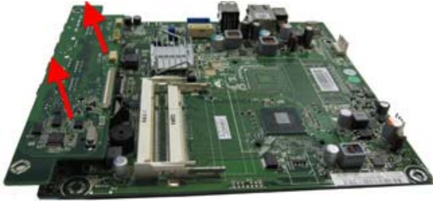
Figure 8-23 Removing the I/O board from the system board
