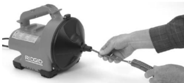
Figure 2 – Feeding Cable into Guide Hose
