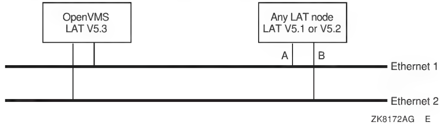
Figure 12-5 Unsupported Multiple Address LAT Configuration
