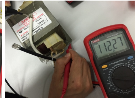
Secondary winding resistance (Scrape the paint on metal base to test)
