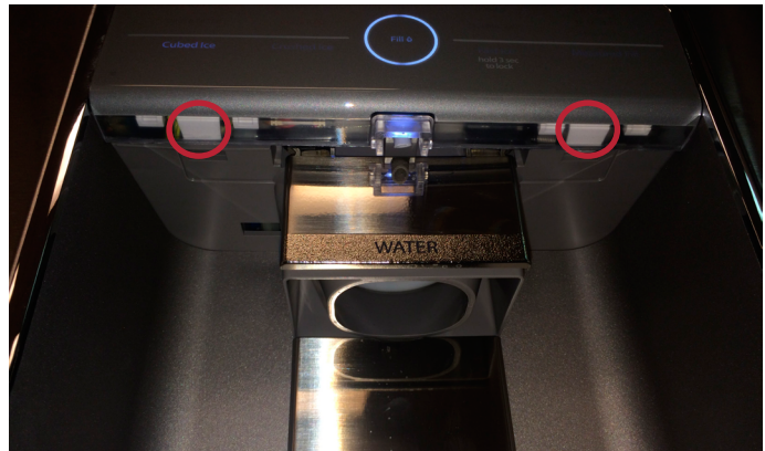
FIGURE 8: Retaining Clips (Circled in Red).
